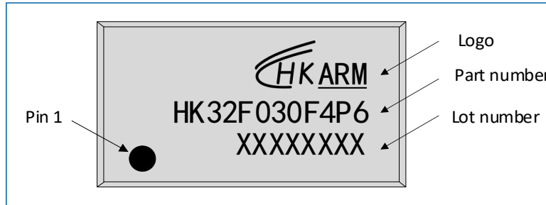
Figure 6-9 TSSOP20 HK32F030F4P6 marking example
